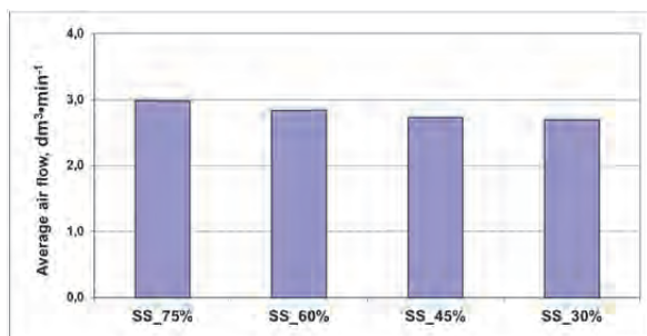
Fig. 6. Average air flow for studied mixtures; SS_75%, SS_60%, SS_45%, SS_30% as in Table 1; source: own study
