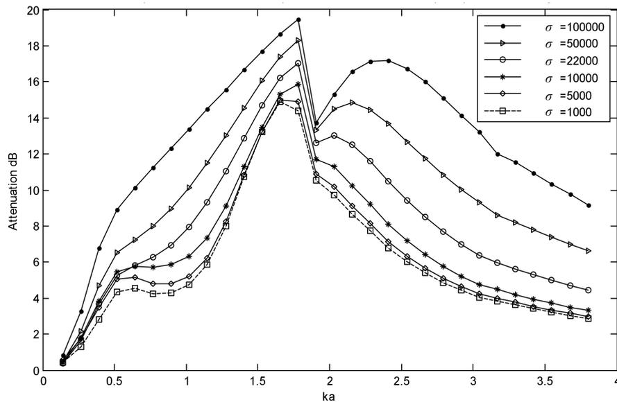
Fig. 7. Effect of the flow resistivity  $\sigma$  [ $\text{Nm}^{-1}\text{s}$ ] of the porous material on the acoustic power attenuation of the lined duct element.
