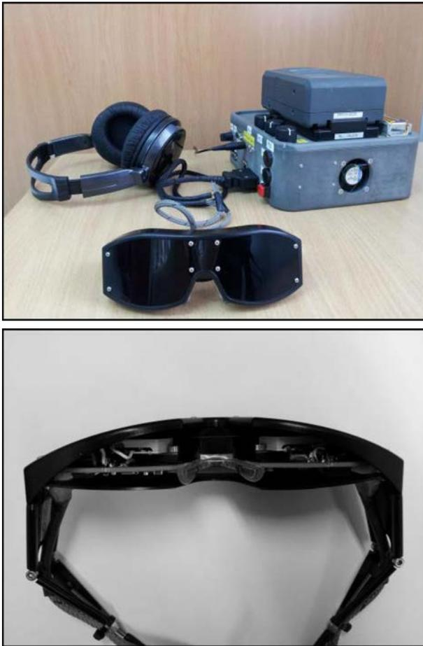
Fig. 2. System components. The laser was assembled on a pair of glasses.
