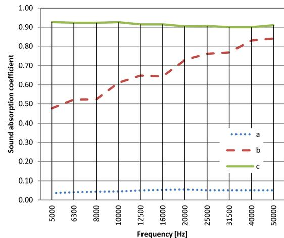
Fig. 8. Sound absorption coefficient of materials in 1/3 octave frequency bands of the test chamber: a – in an empty chamber (wood), b – with polyurethane foam, c – with mineral wool.
