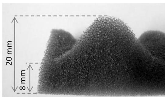
Fig. 2. Examined materials – the polyurethane foam.
