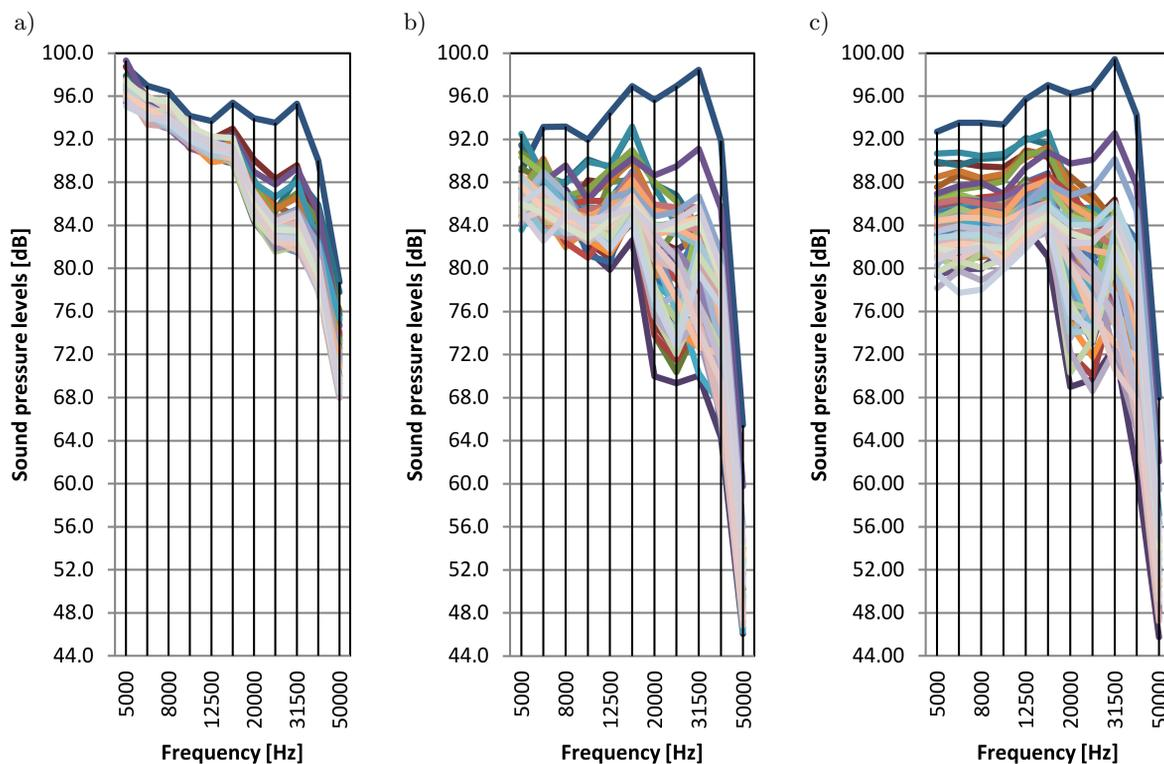
Fig. 3. Sound pressure levels in 1/3 octave frequency bands in the test chamber in a steady state: a) in an empty chamber, b) with polyurethane foam (Fig. 2), c) with mineral wool 50 mm, for 64 measurement point.
