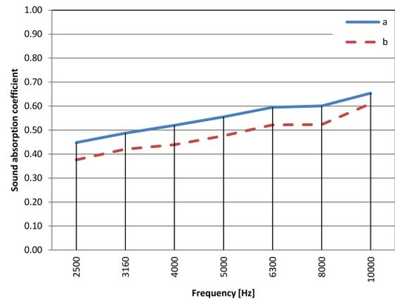
Fig. 7. Sound absorption coefficient of a material made of polyurethane foam in the frequency band 2 500–10 000 Hz: a – defined in a reverberation chamber in standard laboratory (volume 200 m<sup>3</sup>), according to the method EN ISO 354:2003, b – defined by means of the suggested method in the test chamber.
