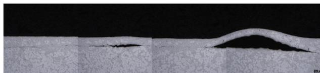
Fig. 4. Clearly visible oxide film between blister layer and the casting, 25x
