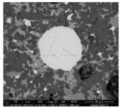
Fig. 1. Planetary arrangement of the copper droplets suspend in the liquid slag; small droplets tend to be swallowed by the dominant copper droplet in order to diminish its surface tension; also rod-like droplets tend to join the dominant droplet, to support a coagulation
