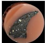
Fig. 2e. Results of the copper droplets coagulation after the St1, St2, R2 (5% of each), and St4 (2%) - chemical treatment performed for 10 minutes
