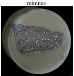
Fig. 2d. Results of the copper droplets coagulation after the St1, St2, (5% of each) and St4 (2%) - chemical treatment performed for 10 minutes
