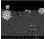
Fig. 3c. Copper droplets localization at the liquid slag's surface; even a distinguished large enough droplet tends towards the liquid slag's surface (not to the crucible bottom), (industrial chemical)
