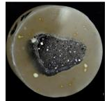
Fig. 2b. Results of the copper droplets coagulation after the St1 and St2 (5% of each) - chemicals treatment performed for 10 minutes
