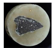
Fig. 2a. Results of the copper droplets coagulation after the St1 (5%) - chemical treatment performed for 10 minutes
