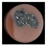
Fig. 2c. Results of the copper droplets coagulation after the St1, St2, and R2 (5% of each) - chemicals treatment performed for 10
