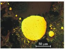
Fig. 3a. Agglomeration of the copper droplets at the liquid slag's surface due to buoyancy force effect on the studied suspension
