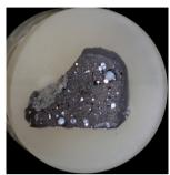
Fig. 2f. Results of the copper droplets coagulation after the St1, St2, St3, and R2 (5% of each) and St4 (2%) - chemical treatment performed for 10 minutes
