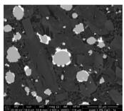
Fig. 3b. Agglomerations of the copper droplets as a positive result of the industrial chemical interaction with the suspension
