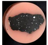
Fig. 2h. Results of the copper droplets coagulation after the R1 (5%) - chemical treatment performed for 20 minutes
