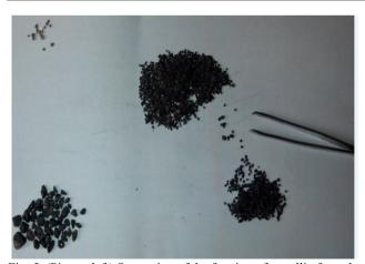
Fig. 5. (Picture left) Separation of the fraction of metallic from the slag: 1 - droplets of copper or a copper alloy drops separated from the slag; 2 - waste slag with copper droplets; 3 - greater fractions were re-fragmentation; 4 - waste slag
