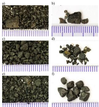
Fig. 7 a, b) Photographs gross fraction of the iron silicate slag-free copper by means of component A; c, d) Macroscopic photographs fraction of the iron silicate slag-free copper by means of component B; e, f) Photographs of gross fraction of the iron silicate slag-free copper by means of component D (scale division correspond with 1 mm)
