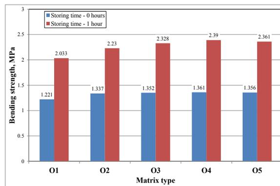
Fig. 7. Bending strength of cores prepared on O1- O5 matrices. Shooting pressure 5 atn.
