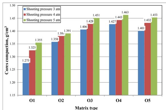
Fig. 9. Influence of the matrix grain size and the shooting pressure on cores compaction
