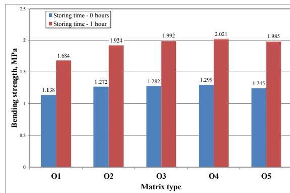
Fig. 6. Bending strength of cores prepared on O1- O5 matrices. Shooting pressure 4 atn.
