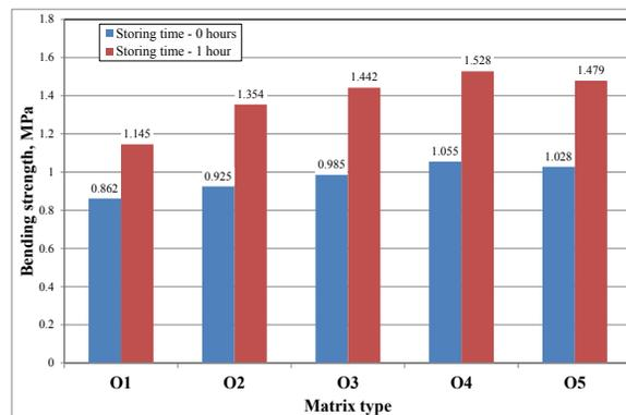
Fig. 5. Bending strength of cores prepared on O1- O5 matrices. Shooting pressure 3 atn.
