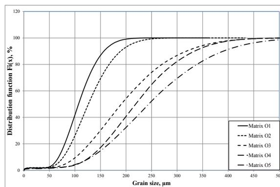
Fig. 2. Distribution function  $F_i(x)$  of grain sizes for matrices O1÷O5
