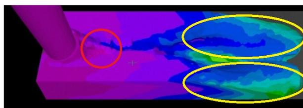
Fig. 7. Filling at the beginning of the runner
