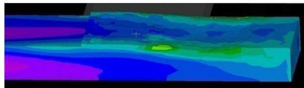
Fig. 11. Filling at the end of the runner
