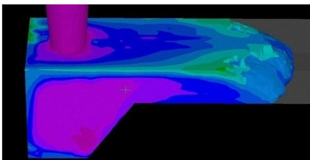
Fig. 10. Filling at the beginning of the runner
