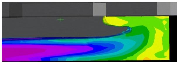
Fig. 4. Filling at the end of the runner
