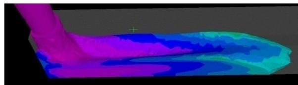
Fig. 2. Filling at the beginning of the runner
