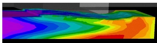
Fig. 8. Filling at the end of the runner
