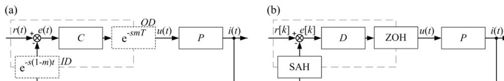
Fig. 3. Control system models structure: a) analog models optionally using delay blocks  $ID$  and  $OD$ ; b) digital models using two different plant  $P$  models
