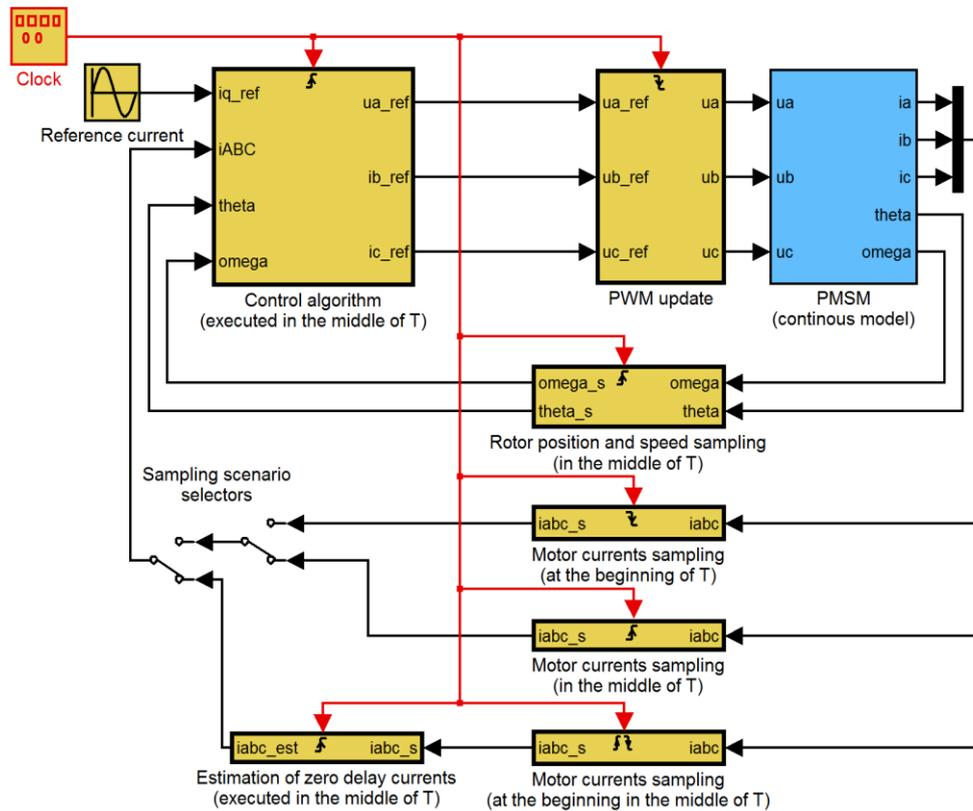
Fig. 4. Reference model of the PMSM drive implemented in Simulink
