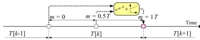
Fig. 2. Timing of digital events in current control cycles for sampling at the beginning of the control cycle ( $m = 0$ ), sampling in the middle of the control cycle ( $m = T/2$ ), and estimating the zero-delay current value ( $m = T$ )
