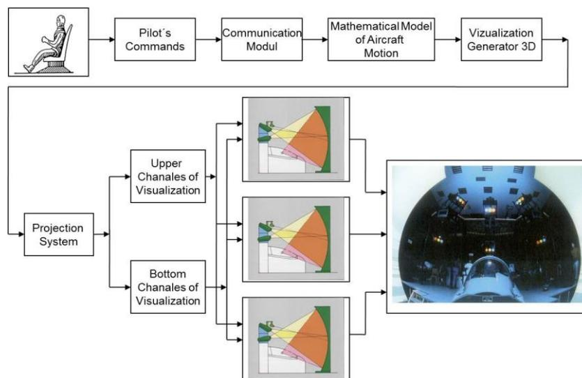
Fig. 2. Principle of a pilot's activity and its visualization in a projection system
