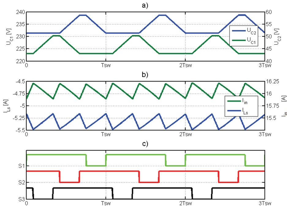
Fig. 3. The steady state CCM waveforms in the DC-DC SEPIC converter with two flying-capacitor cells: the flying capacitors voltages ( $u_{C1}$ ,  $u_{C2}$ ), inductors currents ( $i_{Lin}$ ,  $i_{Ls}$ ), power switches control signals ( $S_n$ );  $U_{out} = 400$  V,  $P_{out} = 2$  kW,  $D = 0.75$  and other of parameters according to Table 1
