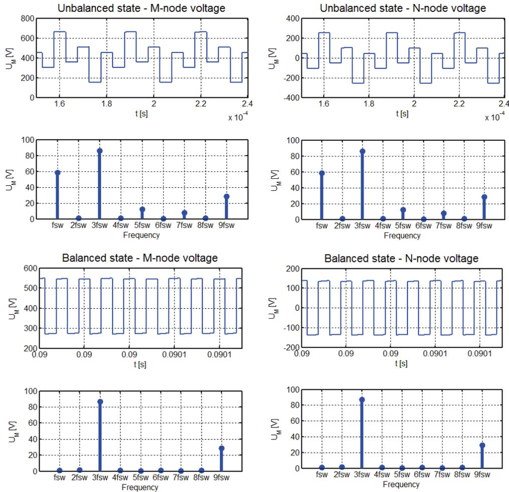
Fig. 6. Voltage in node  $M$  and  $N$  under the balanced and unbalanced state presented in time and frequency domain.  $U_{out} = 400$  V,  $P_{out} = 2$  kW ( $R_d = 78.8 \Omega$ ),  $D = 0.5$ . Matlab/Simulink simulation results
