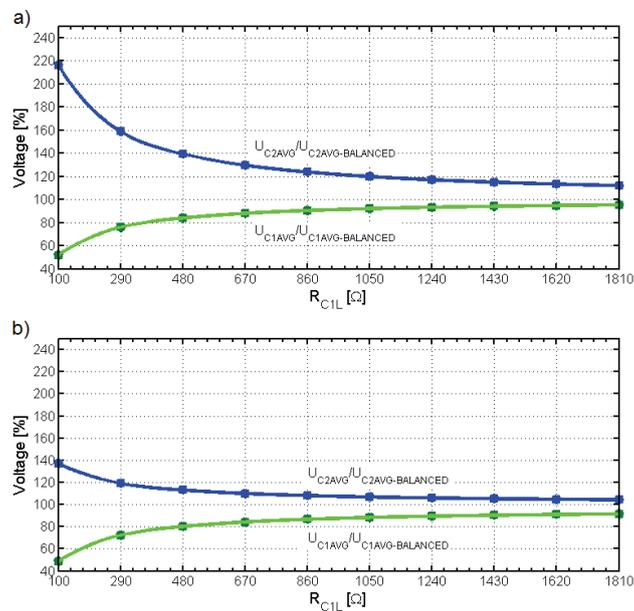
Fig. 8. Balancing effectiveness for two different balancer resistance: a)  $R_b = 300 \Omega$ , b)  $R_b = 50 \Omega$ .  $R_{C1L}$  is leakage resistance parallel connected to capacitor  $C_1$ .  $U_{out} = 400$  V,  $D = 0.5$ ,  $P_{out} = 2$  kW ( $R_d = 78.8 \Omega$ ). Matlab/Simulink simulation results
