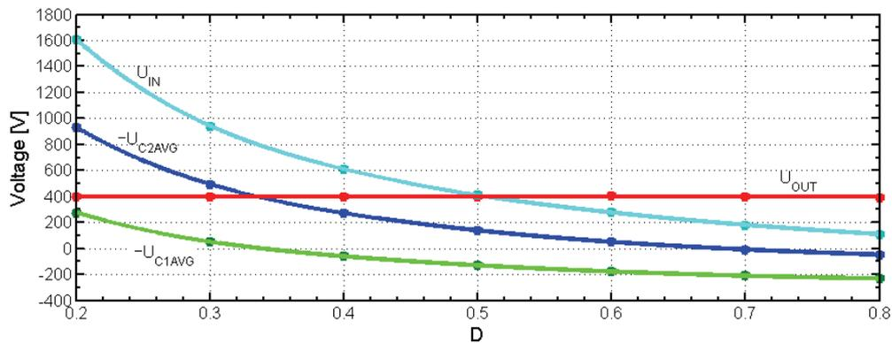
Fig. 4. The average voltage measurements of the flying-capacitors DC-DC converter vs. duty cycle ( $D$ ) for  $U_{out} = \text{const} = 400 \text{ V}$ ,  $P_{out} = 2 \text{ kW}$  ( $R_d = 78.8 \Omega$ ). CCM operation. Matlab/Simulink simulation results
