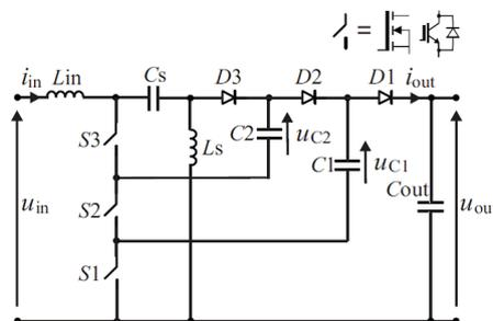
Fig. 1. The DC-DC SEPIC converter with two flying-capacitor cells
