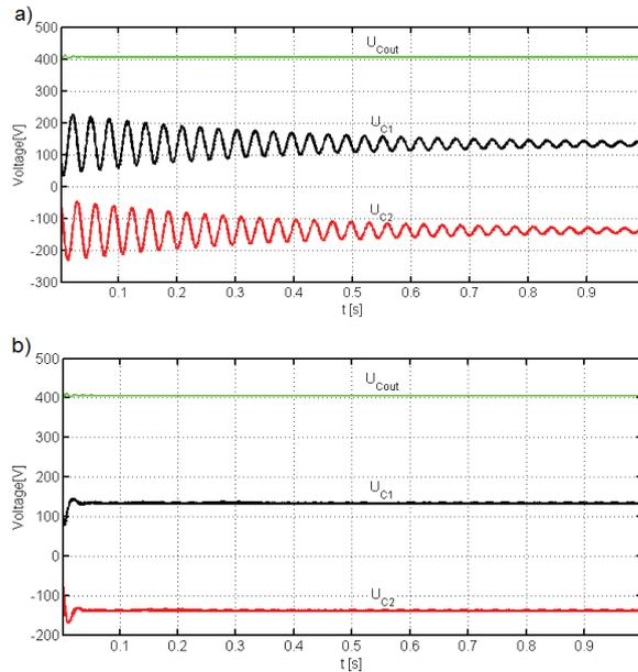
Fig. 7. The voltage across flying-capacitors and output voltage during a balancing process: a) caused only by the natural converter current, b) with the injected balancing current  $i_b$ ;  $D = 0.5$ ,  $P_{out} = 2$  kW ( $R_d = 78.8 \Omega$ ). CCM operation. Matlab/Simulink simulation results
