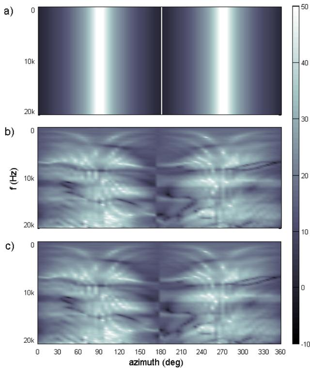
Fig. 7. ILD azimuth functions. The gray map describes frequency dependence of ILD across positions of AP (a), HRTF (b), and Differential HRTF (c) positioning methods for the range of  $360^\circ$  in the horizontal plane. The bar corresponds to the magnitude in dB.
