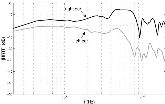
Fig. 2. HRTF magnitude. The magnitude of the HRTF of an artificial head (ALGAZI *et al.*, 2001) for  $\vartheta = 70^\circ$  and  $\varphi = 0^\circ$ . Spectral peaks and notches vary uniquely in accordance with the source position.
