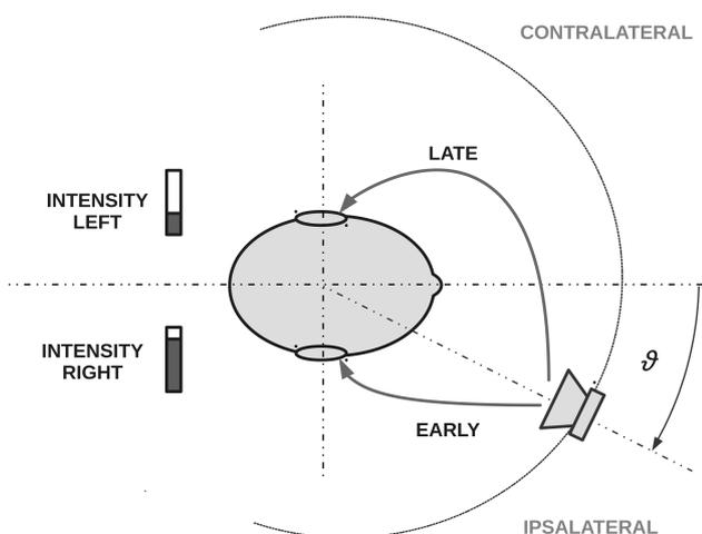
Fig. 1. ILD, ITD, and azimuth. A schematic top view of the spatial arrangement of the listener and sound source. Azimuth  $\vartheta$  is measured from the eye-view. Higher sound intensity and early sound arrival are on the right side.
