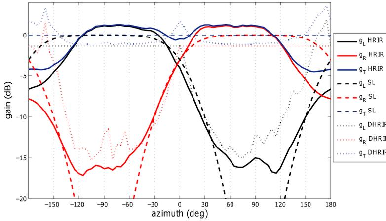
Fig. 5. Azimuth related gains of AP, HRTF, and DHRTF. Logarithmic expressions of channel gains are shown here for the three compared methods. Gains of the left,  $g_L$ , and right,  $g_R$ , channels are shown together with the total gain  $g_T = g_L + g_R$ . Solid lines show HRIR gains of the HRTF, dashed lines show sine law gains of the AP, and dotted lines show DHRIR gain of the DHRTF method.
