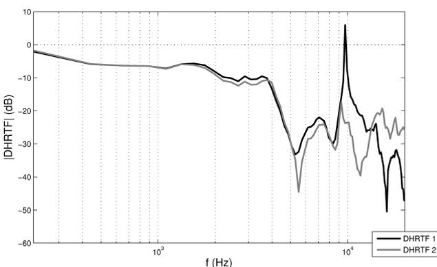
Fig. 4. DHRTF magnitude. The DHRTF for a source placed in the horizontal plane ( $\vartheta = 70^\circ$  and  $\varphi = 0^\circ$ ) is created from two different sets (different subjects) of HRTF. The presence of the spectral spike (black line) exceeding the level of 0 dB is undesirable due to the occurrence of positioning artifacts. The DHRTF represented by gray line is not subject to artifacts.
