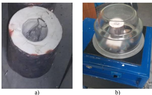
Fig. 2. Vacuum pressure infiltration: a) plaster mould, b) view of infiltration equipment
