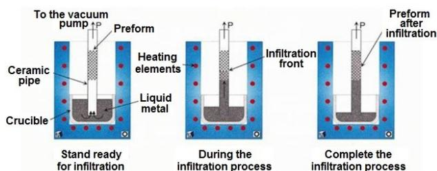
Fig. 1. Schema of vacuum pressure infiltration [4]
