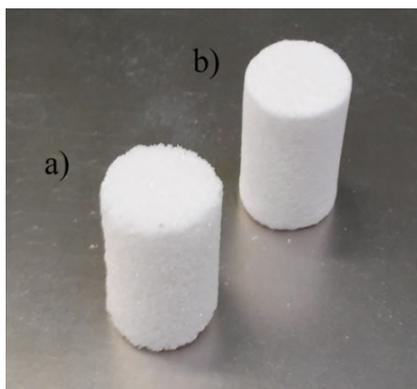
Fig. 4. Reinforcement preforms a) FEPA 046, b) FEPA 100
