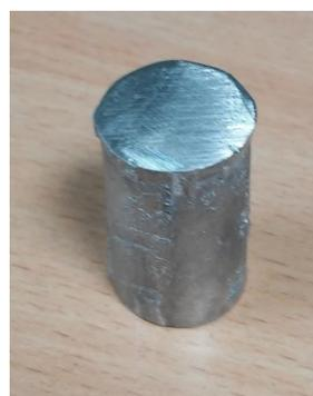
Fig. 3. Composite cast  $\phi=20\text{mm}$ ,  $h=30\text{mm}$ : matrix TBC20, reinforcement sinter alumina powder
