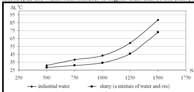
Fig. 3. The dependence of temperature on the number of electrical discharges in different media: 1 – industrial water;
