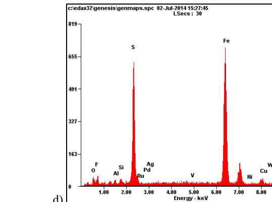
Fig. 5. Microstructures and energy-dispersive spectra of the Akbastau ore: a, c - after mechanical crushing; b, d - after electric pulse reduction
