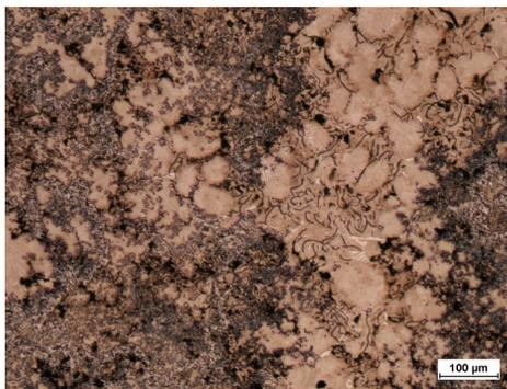
Fig. 5. Microstructure of surface layer of casting reinforced by Ti insert, etch. Nital, mag. 100x., LOM
