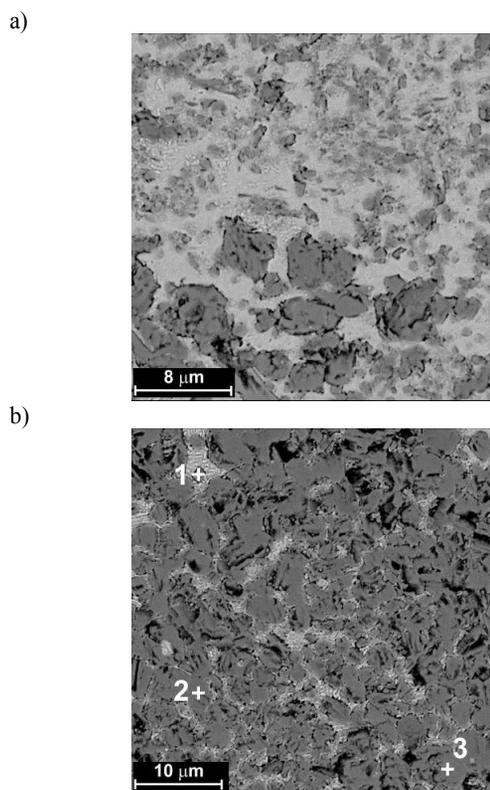
Fig. 6 Microstructure of surface layer of casting reinforced by titanium carbides, SEM
