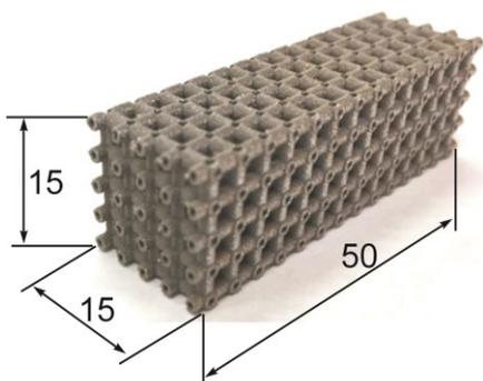
Fig. 1. Scaffold insert made from pure Ti powder
