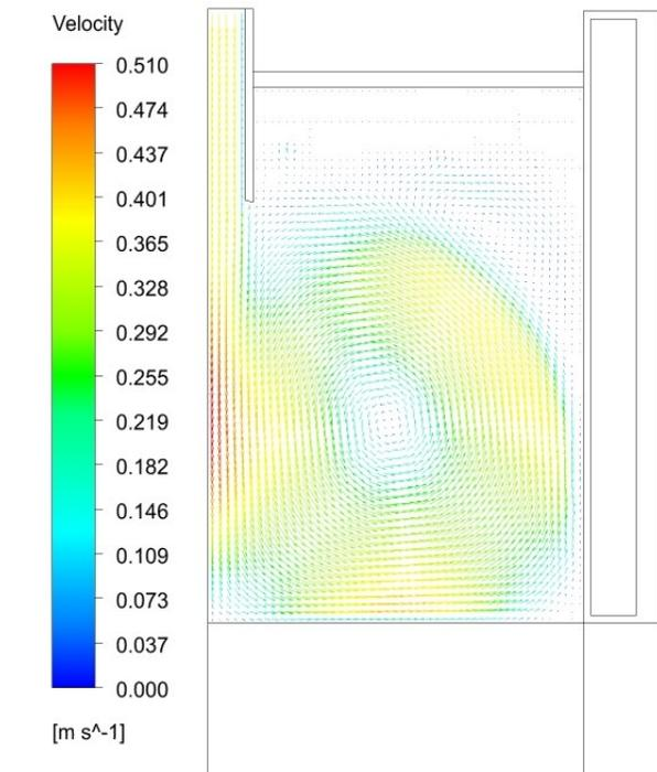
Fig. 3. Velocity field after filling of the continuous casting mould at time  $t=20$  s, I variant
