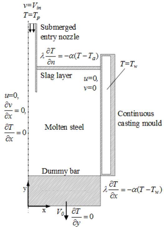
Fig. 1. Schematic illustration of the continuous casting mould containing boundary conditions
