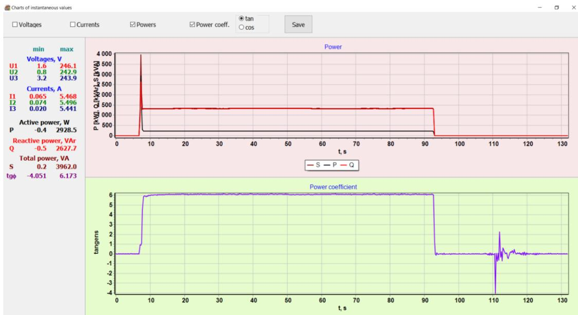
Fig. 8. The diagram of changes in active, passive, apparent power consumption and  $\text{tg}\phi$  power factor in supply system of a model vibratory unit without the inverter at the frequency of 50 Hz
