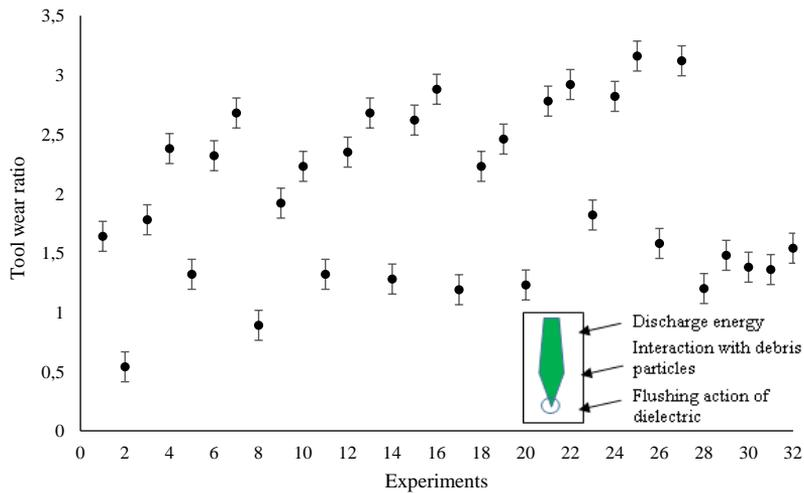
Fig. 2. The data of tool electrode wear ratio for all the experimental trials and an illustration of the causes of tool wear in the micro-EDM process
