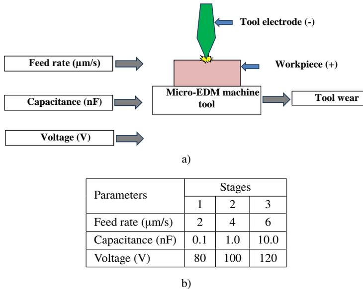
Fig. 1. a) A schematic of the basic experimental set-up [29] for evaluating the effect of micro-EDM inputs illustrating the methodology, b) stages and parameters of the experiments
