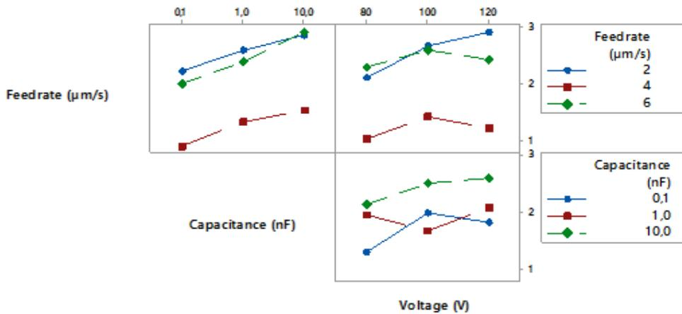
Fig. 6. Interaction effects on the tool wear ratio (interactions: feed rate  $\times$  capacitance, voltage  $\times$  capacitance and feed rate  $\times$  voltage)
