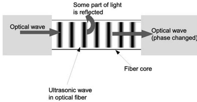
Fig. 1. Periodic change of the refraction index in optical fiber caused by ultrasonic wave.
