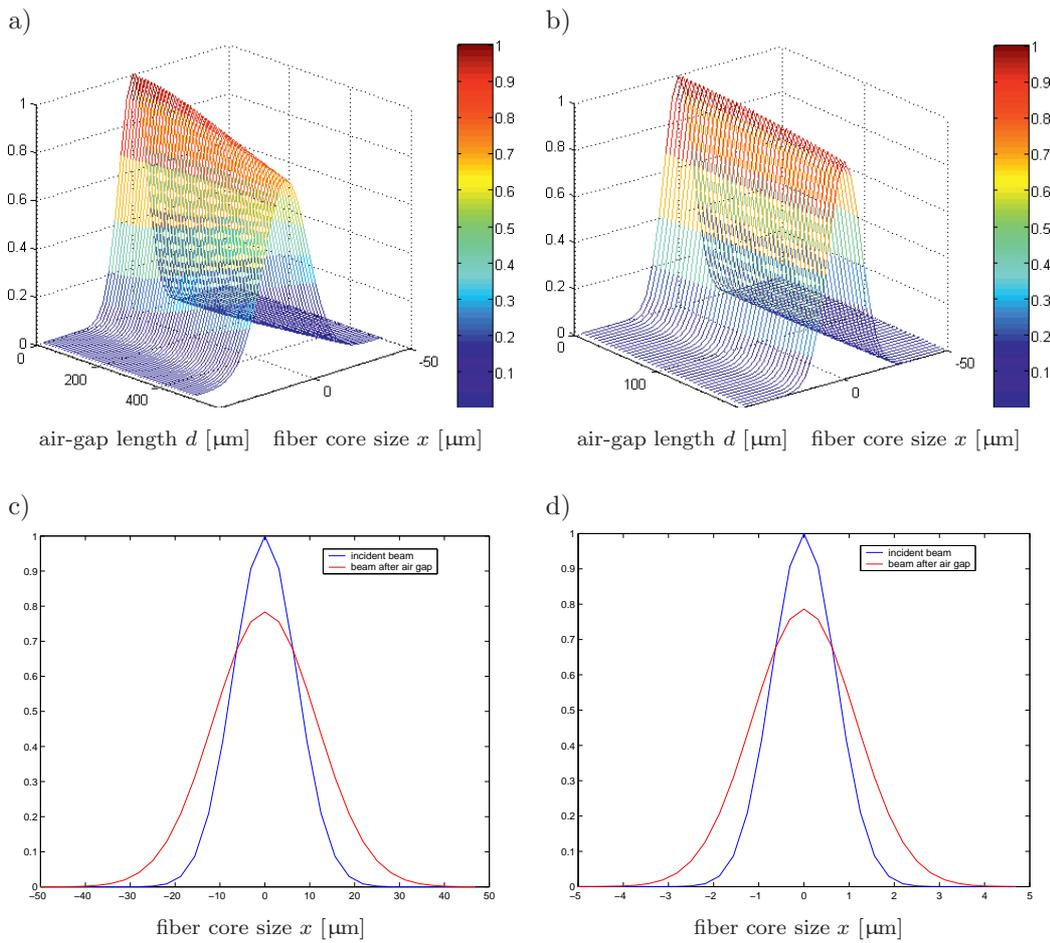
Fig. 4. Influence of the air-gap length on the intensity of the optical wave: a) 3D chart, gap = 500 μm, optical fiber core diameter = 100 μm, b) 3D chart, gap = 200 μm, optical fiber core diameter = 100 μm, c) 2D chart, gap = 500 μm, core diameter = 100 μm, d) 2D chart, gap = 500 μm, core diameter = 10 μm.
