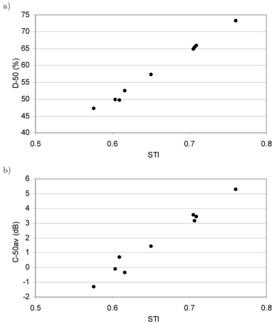
Fig. 1. Relationships between STI mean values and the other measured physical intelligibility parameters: a) Definition (D-50), b) Average Speech Clarity (C-50av).
