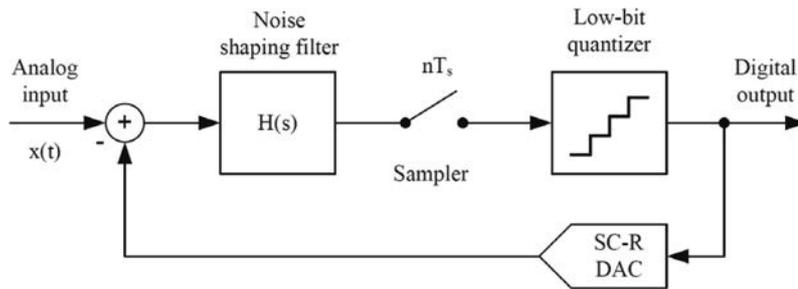
Fig. 10. CT  $\Sigma\Delta$  modulator with SC-R DAC feedback.
