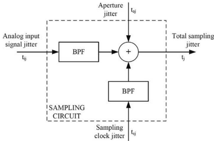
Fig. 6. The total sampling jitter estimation model.
