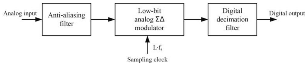
Fig. 2. Block diagram of the  $\Sigma\Delta$  ADC ( $L$  – oversampling ratio).
