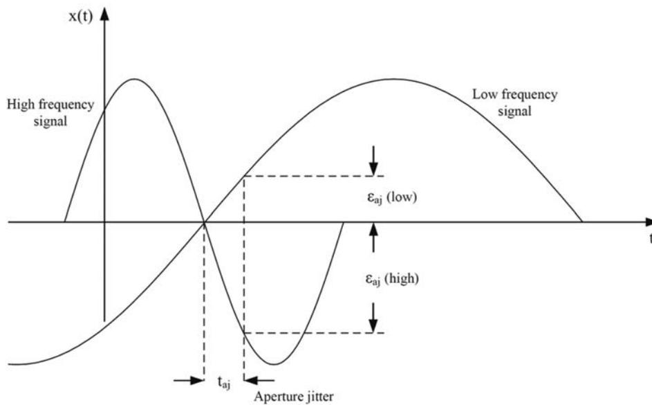
Fig. 5. Voltage error  $\varepsilon_{aj}$  due to aperture jitter  $t_{aj}$ .
