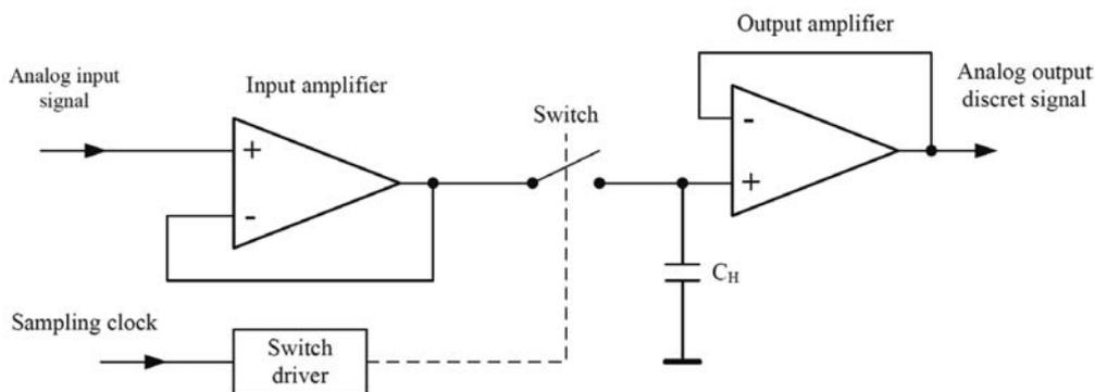
Fig. 3. Simplified model of sample-and-hold amplifier.
