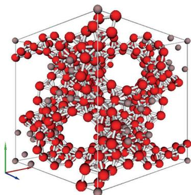
Fig. 1. NaY zeolite structure with cages and channels
