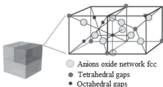
Fig. 1. Crystal structure of spinel [21]
