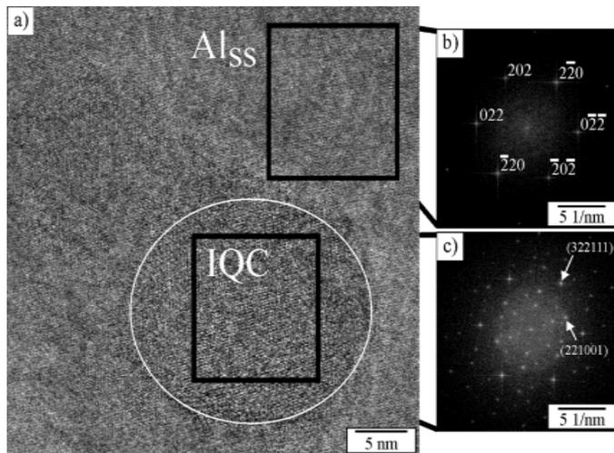
Fig. 6. The HRTEM micrograph of an IQC-precipitate (encircled) within  $Al_{ss}$  with corresponding FFTs for the matrix (zone axis  $[111]$ ), and IQC-precipitate (a threefold zone axis  $[\tau^{-2} 1 0]$ )
