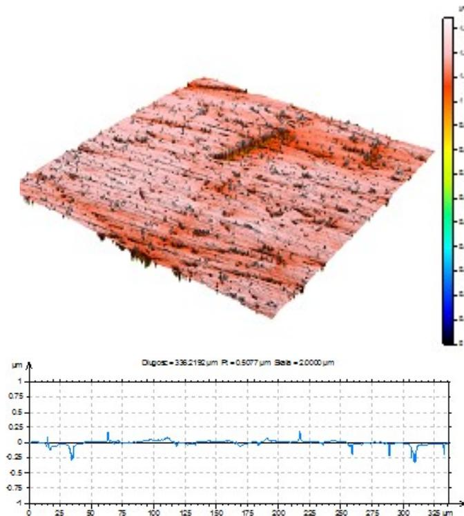
Fig. 4. HS6-5-2C steel disc with an a-C:H coating: a) surface texture, b) roughness profile
