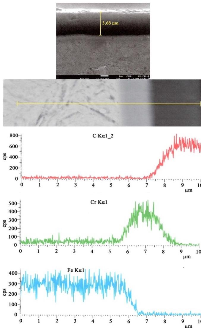
Fig. 2. a) SEM cross section and b) EDS analysis of the a-C:H coating
