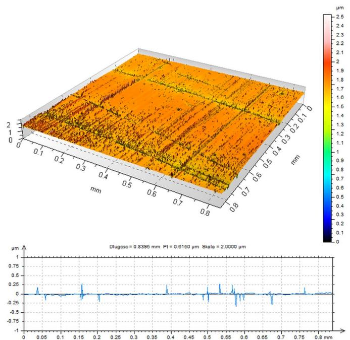
Fig. 12. Surface texture of an a-C:H coating in lubricated contact with an HS6-5-2C steel pin: a) surface topography, b) roughness profile. T-17 tester
