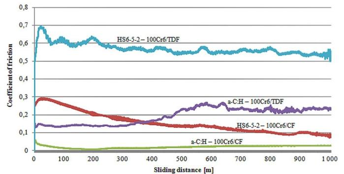
Fig. 5. Coefficient of friction for the HS6-5-2C steel-100Cr6 steel and a-C:H coating-100Cr6 steel systems. Sliding distance:  $s = 1000$  m. Load:  $P = 10$  N. T-01M ball-on-disc tester
