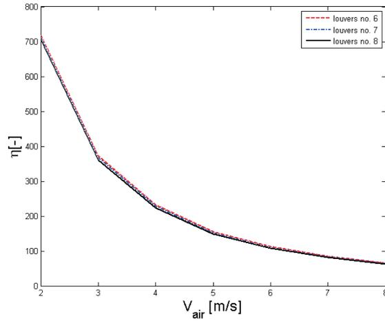
Figure 11: Maximum performance as a function of frontal air velocity for selected geometries.
