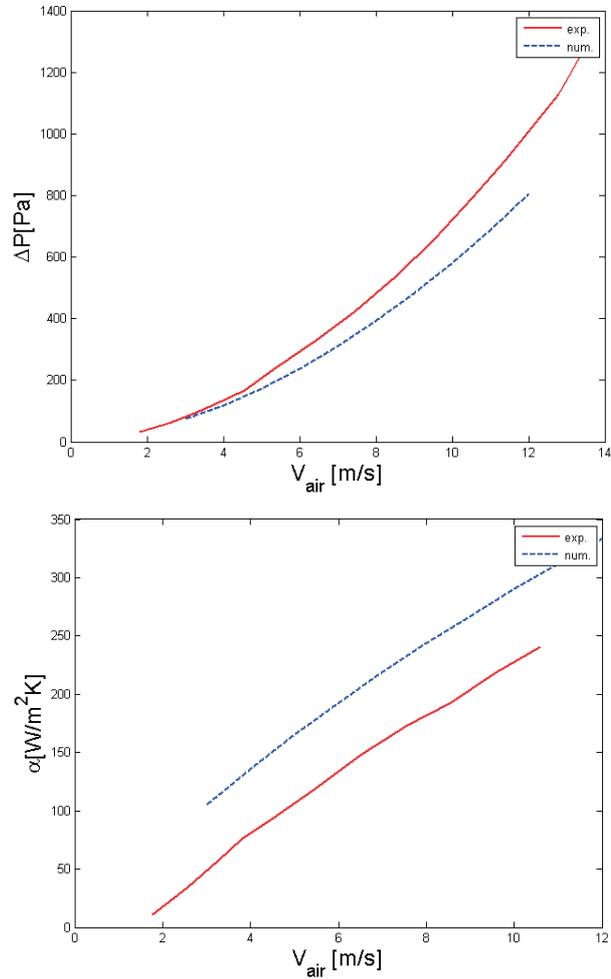
Figure 4: Experimental data by Dong *et al.* [10], compared to corresponding numerical data.
