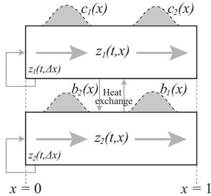
Fig. 1. Parallel-flow heat exchange process
