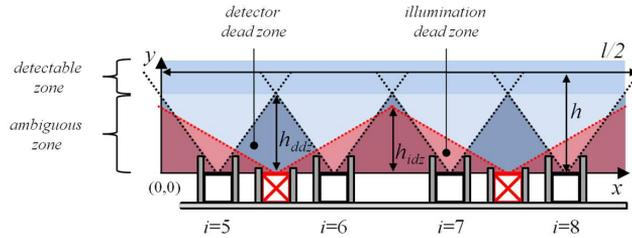
Fig. 3. A sketch of the right side of the sparse optical sensor with three types of zones marked.
