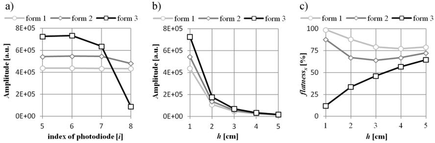
Fig. 10. Strength of the reflected light signals with a 2FJ positioned over a given photodiode at  $h = 1$  cm (a). Strength of the reflected light signals from  $i=5$  photodiode as a function of  $h$  (b). Flatness<sub>x</sub> functions composed of individual flatness<sub>x</sub> values (c).
