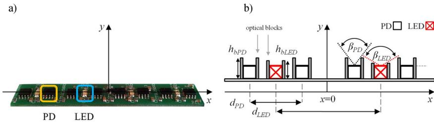
Fig. 1. An optical gesture sensor (without optical blocks for better clarity) (a).
