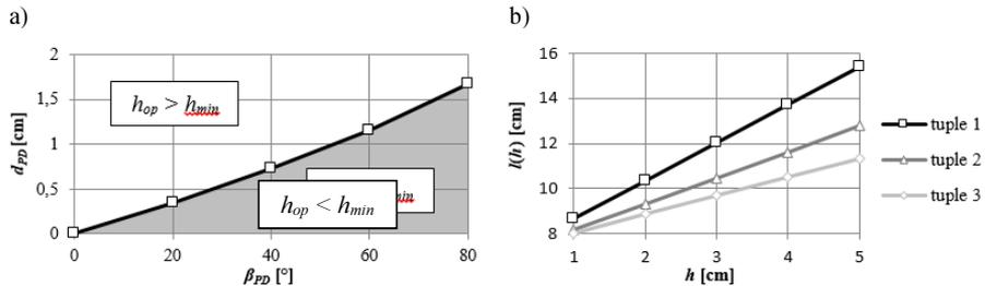
Fig. 11. A function binding values of  $\beta_{PD}$  and  $d_{PD}$  to keep  $h_{op}$  at a proper level (painted area) (a). The values of  $l(h)$  for three different configurations of the sensor, described by three triples (b).
