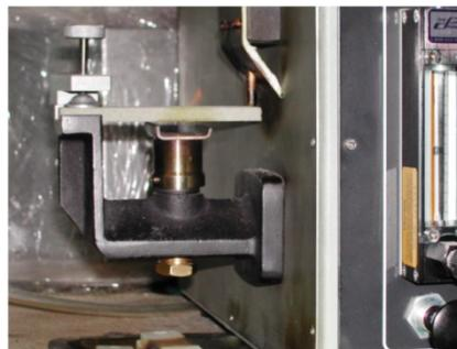
Fig. 2. Measurement module of the BCIRA test apparatus
