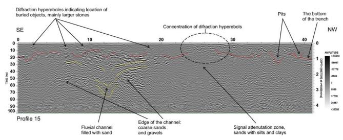
Fig. 13. Interpretation of the GPR reflection profile no. 15 in a central part of the Radomno hillfort.
