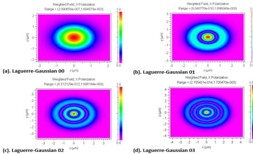
Fig. 2. Four Laguerre-Gaussian over FMF based on SDM.
