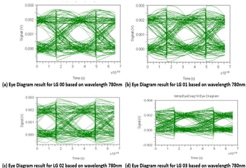
Fig. 8. Eye Diagram result of four LG modes for the wavelength 780 nm.
