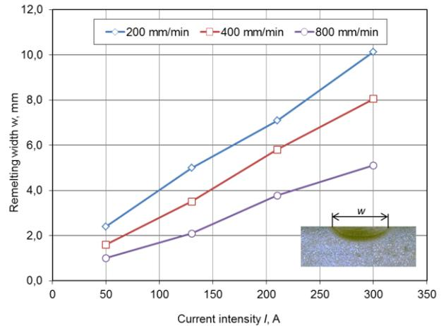
Fig. 4. The effect of the electric arc current intensity and the electric arc scanning speed on width of remeltings made on a plate cast from nodular cast iron
