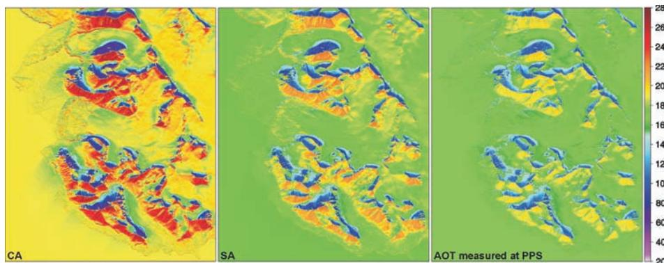
Fig. 4. Modelled incoming total solar radiation for constant (CA), modelled (SA) and measured aerosol optical thickness. All maps are for 2 May 2006.
