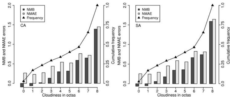
Fig. 7. Normalized Mean Bias (NMB) and Normalized Mean Absolute Error (NMAE) for different low and middle level cloudiness conditions (in octas, cumulative frequency).
