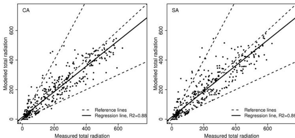
Fig. 5. Modelled vs measured total solar radiation ( $W\ m^{-2}$ ) for cloudiness  $< 2$ . 1:1, 2:1 and 1:2 lines (dashed) and regression line (solid) are given for clarity.
