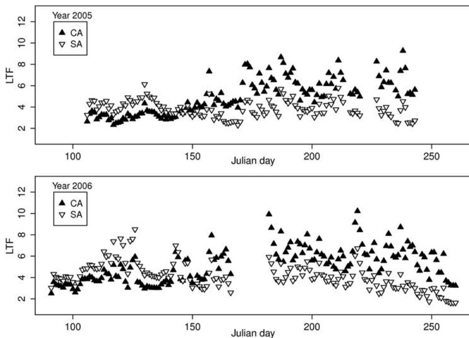
Fig. 3. Daily average Linke Turbidity Factor (LTF) for constant (CA) and modelled aerosol optical thickness (SA).
