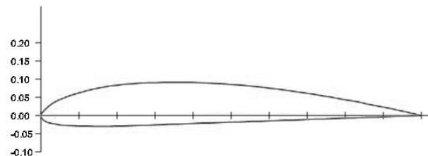
Fig. 5. Geometry of aerofoil profile CLARK Y [21]
