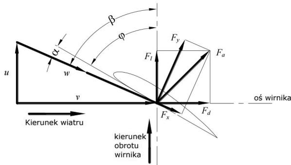
Fig. 1. Forces generated in an aerodynamic profile [6]
