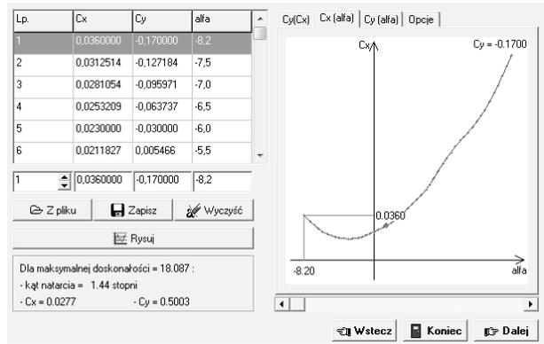
Fig. 7.  $C_x(\alpha)$  characteristics – WIATRAK 1.1 software [own elaboration]
