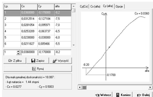
Fig. 8.  $C_y(\alpha)$  characteristics – WIATRAK 1.1 software [own elaboration]
