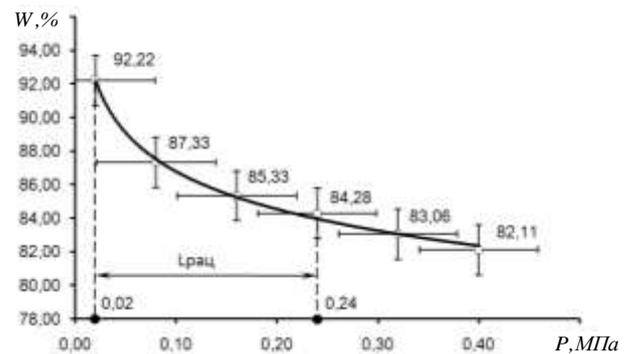
**Fig. 1.** Dependence of lake sapropel humidity changes *W* of pressure on the sample surface *P*
