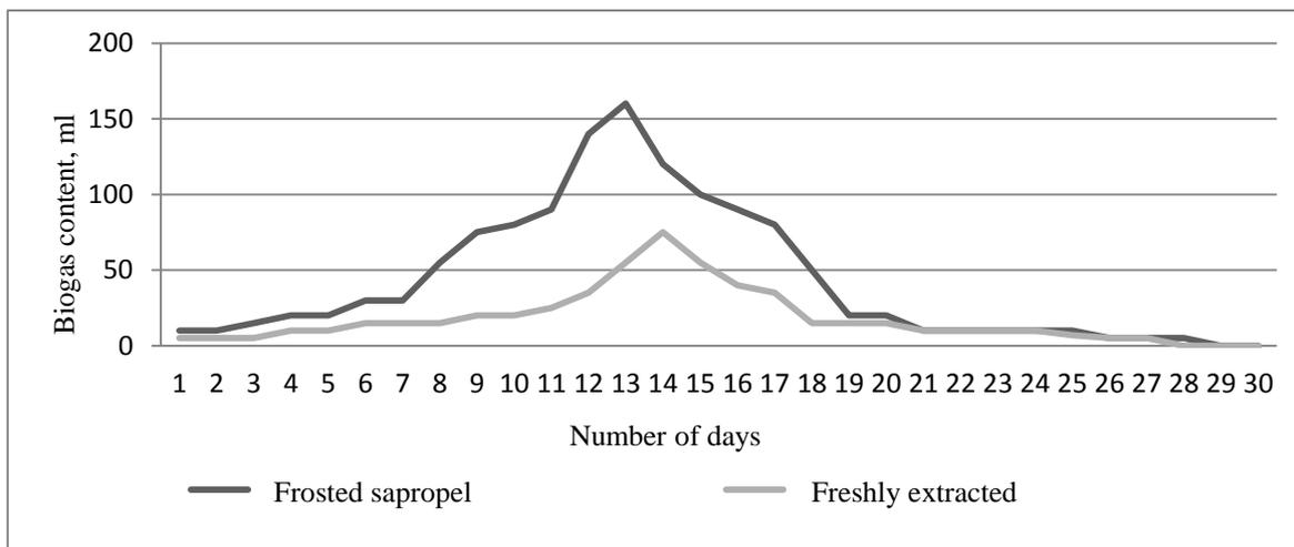
Fig. 3. Biogas emission during fermentation in the laboratory
