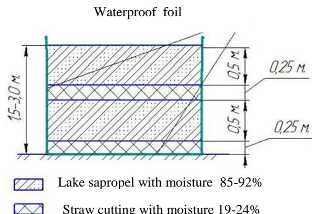
**Fig. 2.** Defining dimensions of collar in composting
