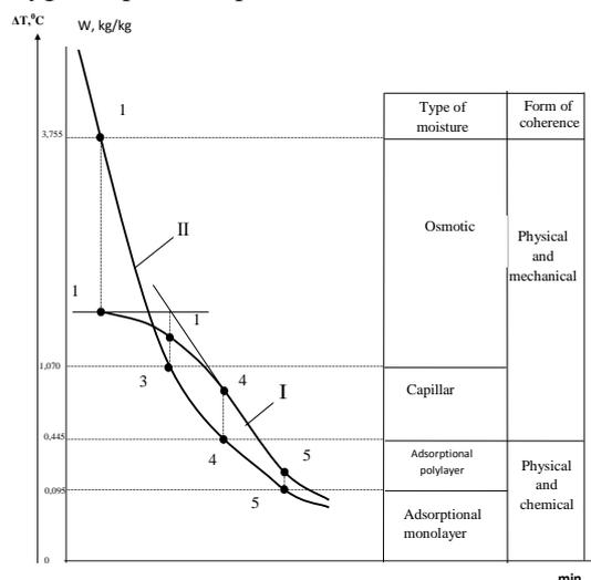
**Fig. 5.** Scheme of moisture removal sequence of various forms of coherence: I - a typical thermogram for a colloidal capillary-porous body; II - experimental curve of organic sapropel drying
