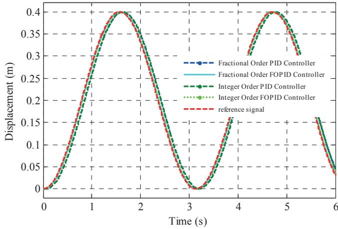
Fig. 10. System responses to sine wave signal
