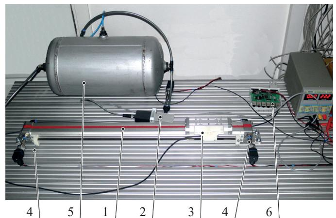
Fig. 1. Test stand for pneumatic drive: 1 – rodless cylinder, 2 – directional control valve, 3 – displacement transducer, 4 – pressure transducers, 5 – pneumatic power supply, 6 – measurement data acquisition system
