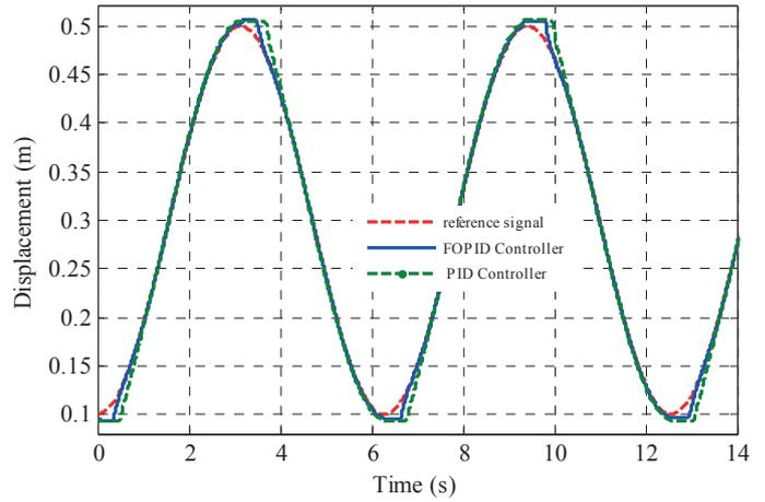
Fig. 13. System responses to sine wave signal
