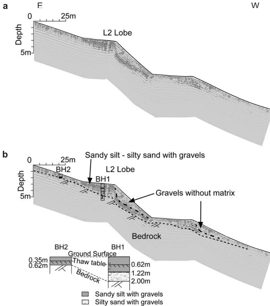
Fig. 5. GPR profile of L2 lobe fitted to the surface topography (a) and its interpretation (b). The positions of boreholes BH1 and BH2 are indicated on the modified GPR profile.
