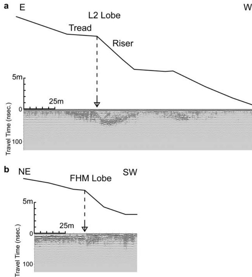
Fig. 4. GPR profiles and surface topography of (a) L2 lobe and (b) FHM lobe. The arrows indicate the corresponding position (top of the frontal riser) on the GPR profiles.
