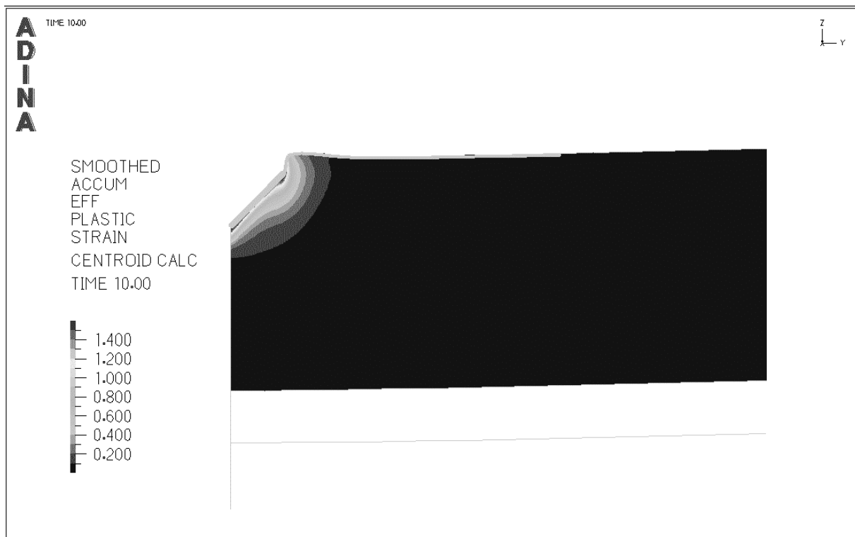
Fig. 9. Strain distribution in the TiN layer for the sharp indenter
