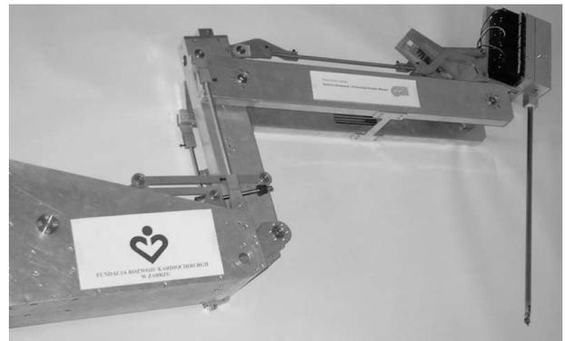
Fig. 2. The arm of the RobIn Heart 0 robot
