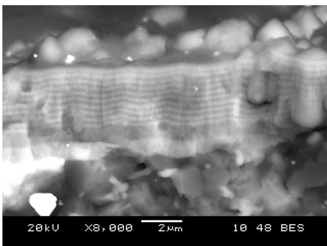
Fig. 2. A SEM micrograph showing the fractured multilayer TiN/(TiAl)N/  $10\times$  (TiN/(TiAl)N) coating deposited on the TACN grade ceramic cutting insert
