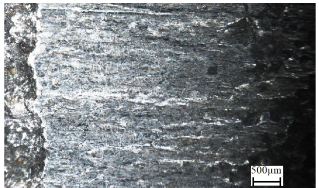
Fig.7. OM image of the surface after AWJ cutting, \times 10
