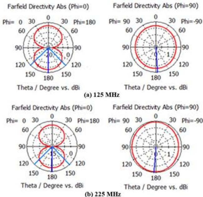
Fig. 8. E-plane and H-plane radiation Patterns at (a) 125 MHz and (b) 225 MHz.
