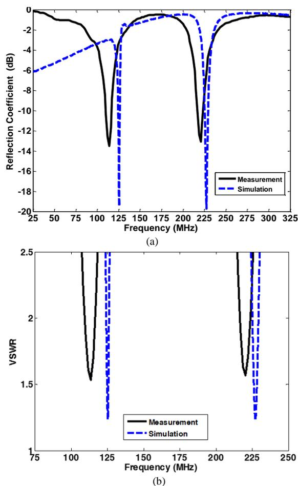
Fig. 10. Measurement versus Simulation Results (a) Reflection coefficient (dB) and (b) VSWR.
