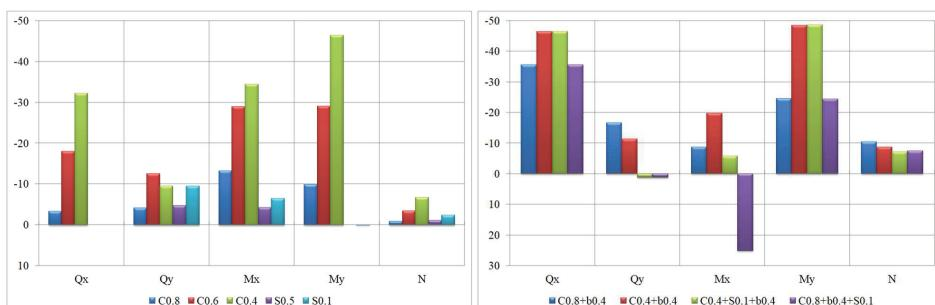
Fig. 9. Percentage ratios of base shear force, base bending moment, and base normal force for the rectangular building (ratio 2.5) with square column cross sections
