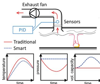
Fig. 2. The concept of the smart smoke control system
