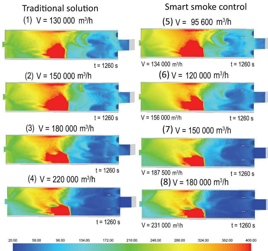
**Fig.4.** The temperature of smoke (20 – 400 °C and more) at the height of 2,00 m above the floor, for four traditional and four smart smoke control systems, as described in [7]. Systems on the right side did operate at approx. 30% lower operating pressure, than their traditional counterparts
