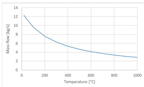
Fig. 3. Change of mass flow rate at exhaust point with capacity of 10 m<sup>3</sup>/s in function of temperature
