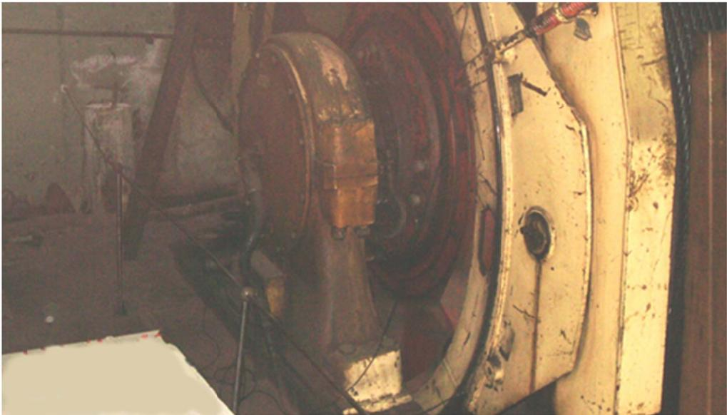
Fig. 1. Brake shoe of a mining hoist 2T3,5X1,7A
