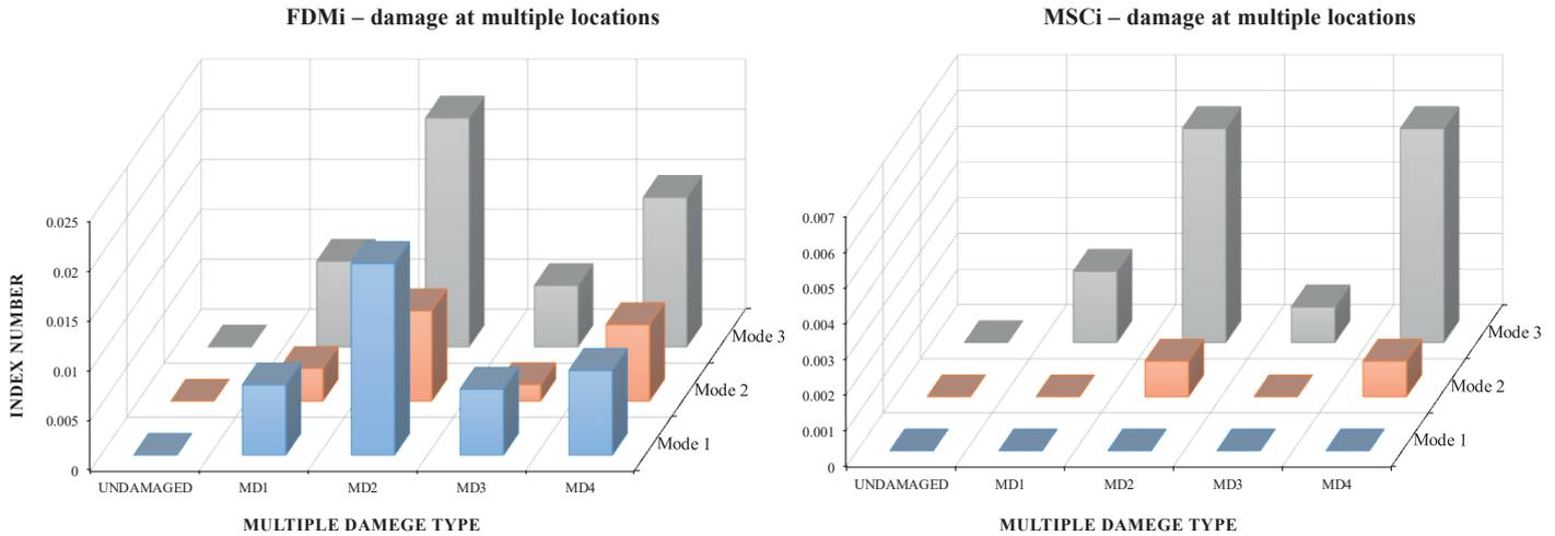
Fig. 11. FDMi and MSCi values comparison for different damage levels and multiple locations
