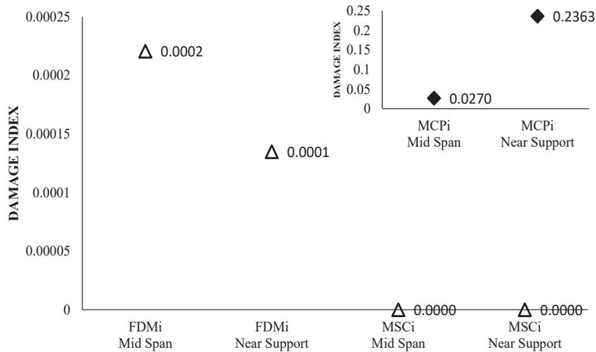
Fig. 9. MCPi comparison with FDMi and MSCi for damage at different locations for 1% ESR
