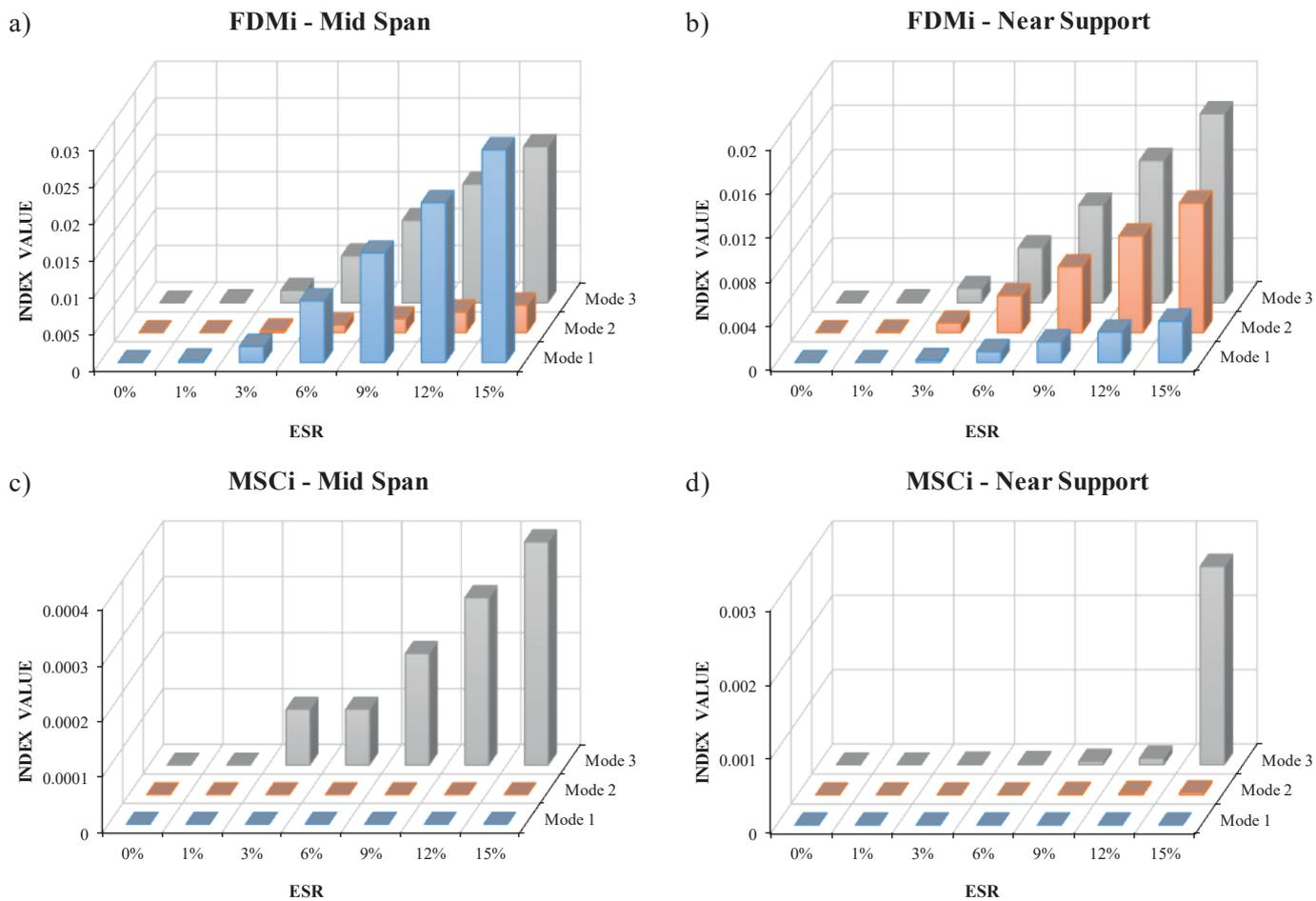
Fig. 7. FDMi and MSCi – comparison for different damage levels and locations
