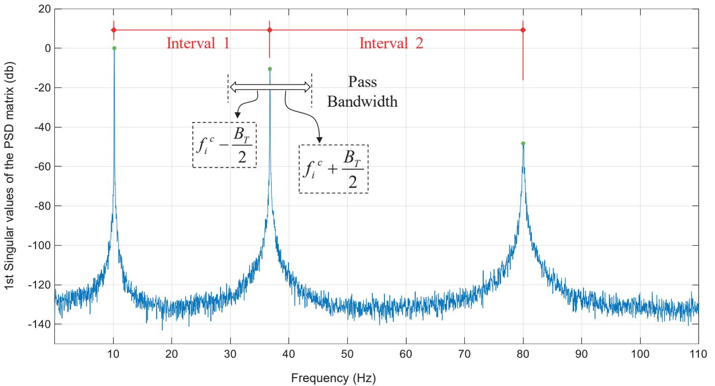
Fig. 1. Selection of pass bandwidth of filter for modal response extraction
