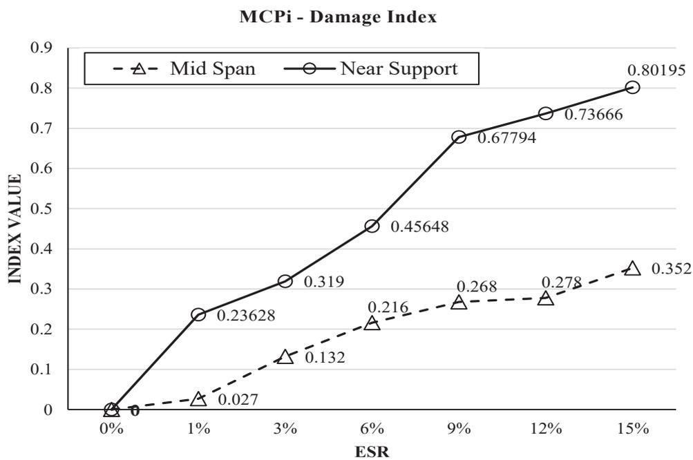
Fig. 8. Comparison of MCPi values for different levels and locations of damage
