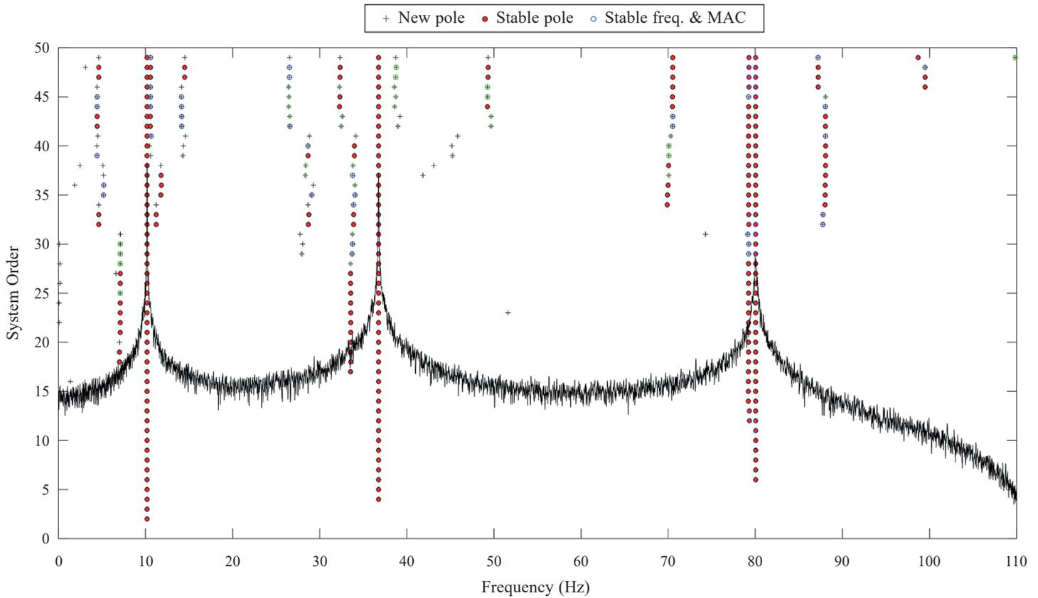
Fig. 6. Stabilization diagram for control beam
