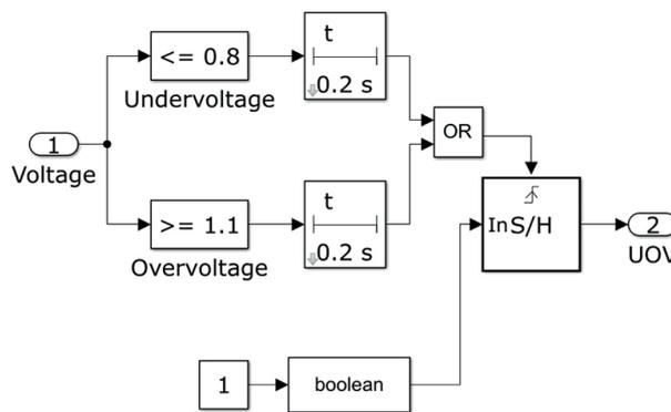
Fig. 5. U/OVP model in Simulink environment
