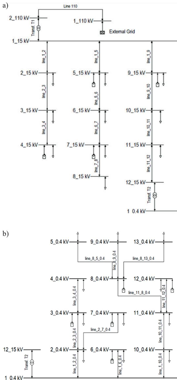
Fig. 1. HV, MV and LV section diagram of the test grid (a – HV and MV section, b – LV section)
