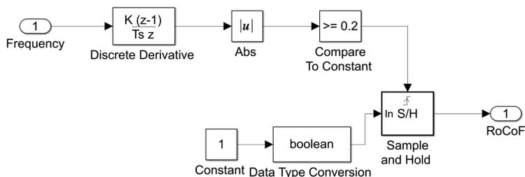
Fig. 6. RoCoF model in Simulink environment
