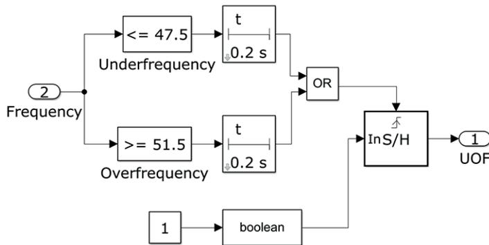
Fig. 4. U/OFP model in Simulink environment
