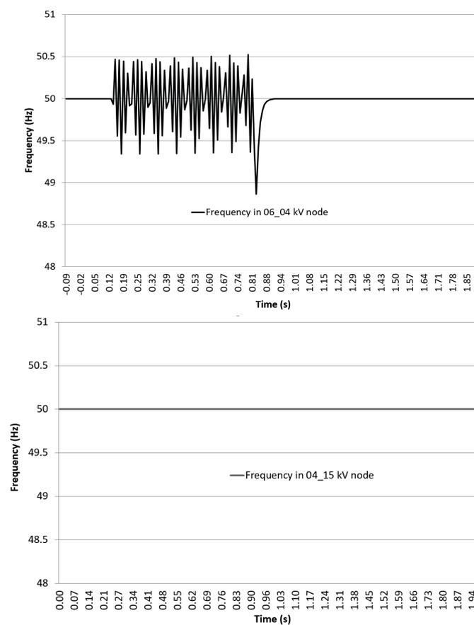
Fig. 2. The example plots of voltage and frequency in selected nodes of the test system. Simulation variant – fault in node 1\_0.4 kV lasting 700 ms.
