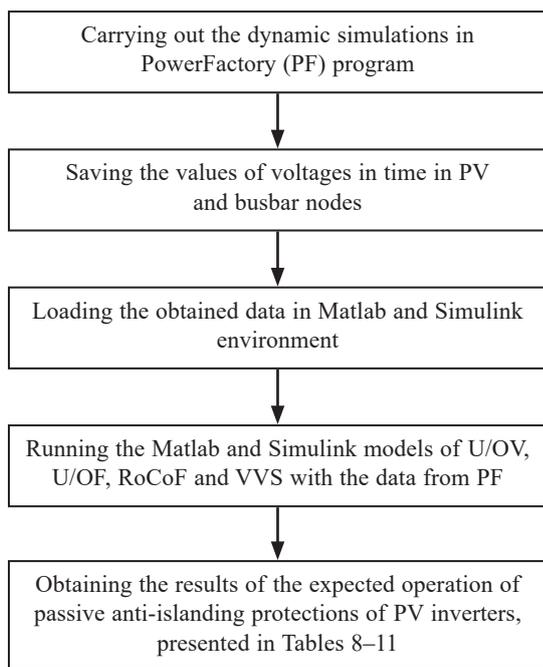
Fig. 3. The actions taken in order to obtain the results of passive anti-islanding protection systems
