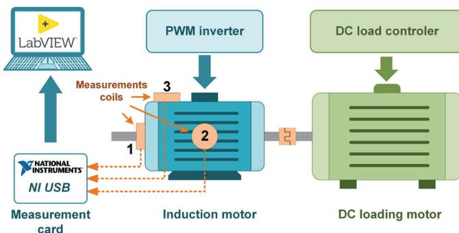
Fig. 6. General scheme of the experimental set-up
