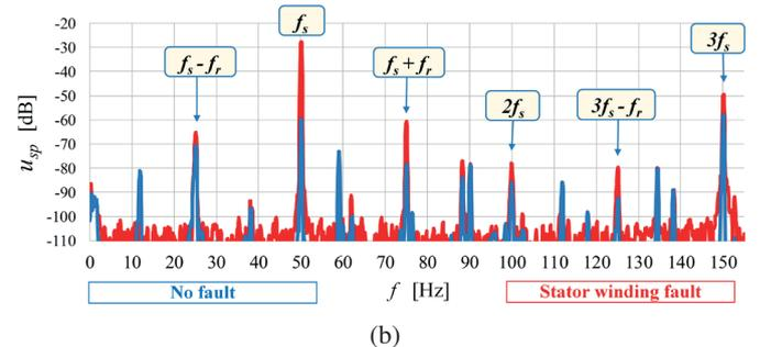
Fig. 3. Axial flux spectrum: (a) for undamaged motor ( $N_{bb} = 0$ ) and with 3 broken rotor cage bars ( $N_{bb} = 3$ ),  $f_s = 50$  Hz,  $T_L = 0.8T_N$ ; (b) for undamaged motor ( $N_{sh} = 0$ ) and with 5 shorted turns in phase A ( $N_{sh} = 5$ ),  $f_s = 50$  Hz,  $T_L = 0.2T_N$
