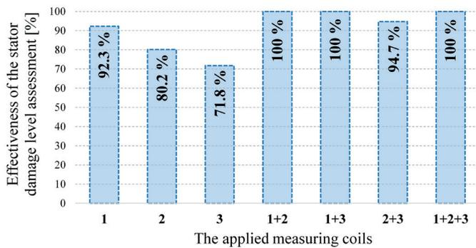
Fig. 10. The influence of the CNN input information to the accuracy of the assessment of stator winding fault level: 1 – measuring coil number one, 2 – measuring coil number two, 3 – measuring coil number three
