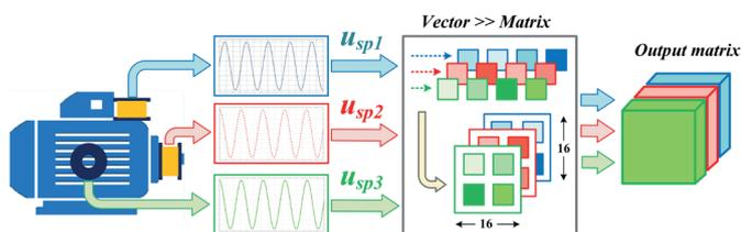
Fig. 4. Elaboration of the input layer of the CNN used for electrical fault detection of the induction motor – idea scheme
