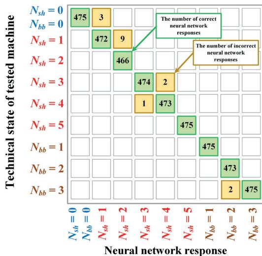
Fig. 8. Convolutional neural network response – CNN-1:  $N_{sh}$  – number of shorted turns in phase A;  $N_{bb}$  – number of broken rotor bars; green envelope – correct neural network responses; yellow envelope – incorrect neural network responses
