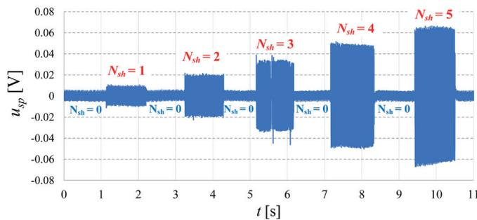
Fig. 2. The influence of the short circuits in the stator winding on the voltage induced in the measuring coil by the axial flux:  $N_{sh}$  – number of shorted turns in phase A,  $f_s = 50$  Hz,  $T_L = 0.1T_N$
