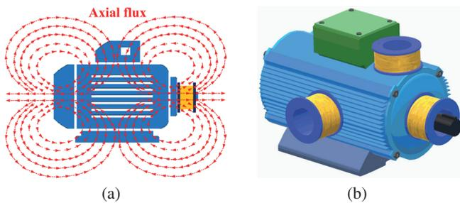
Fig. 1. External stray (axial) flux in a squirrel-cage induction motor (a) and method of placement of axial flux measuring coils (b)
