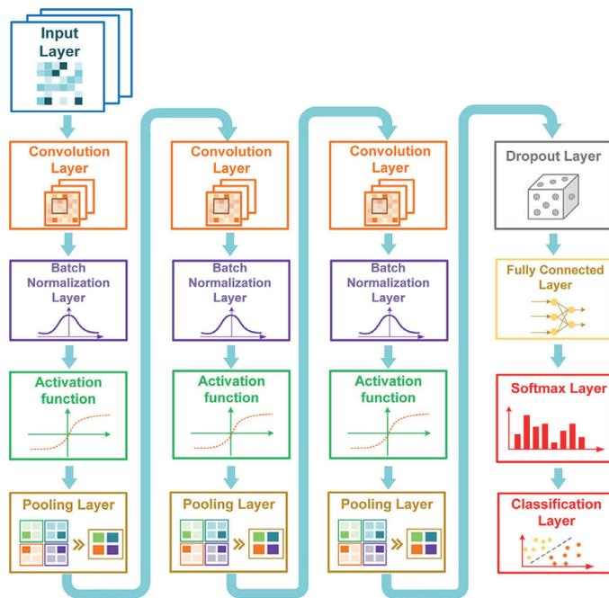
Fig. 5. Developed convolutional neural network structure
