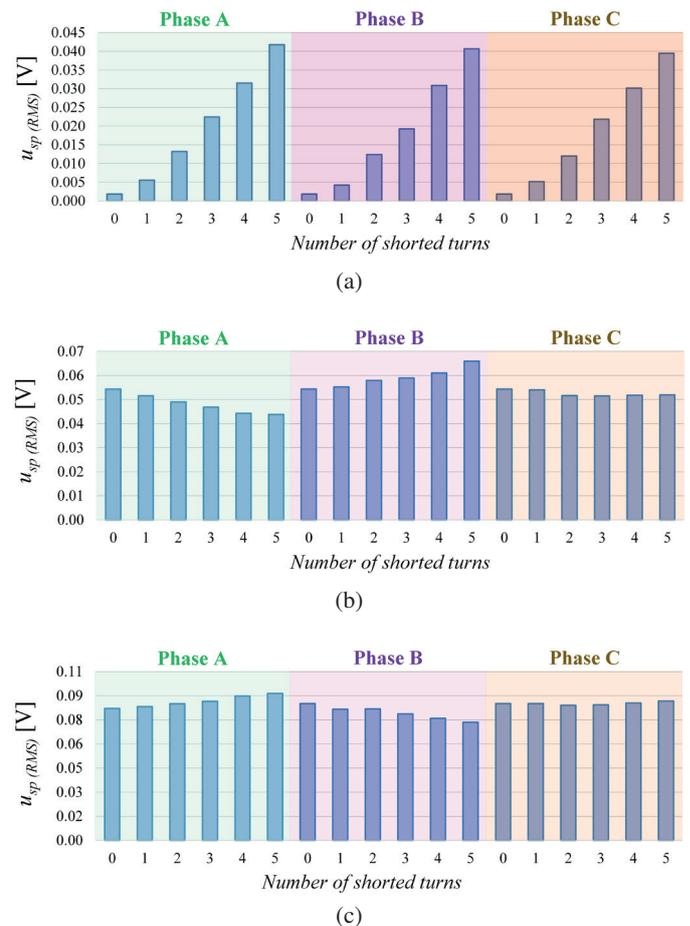
Fig. 9. Influence of shorted turns in stator on the values of the voltages induced in measuring coils: (a) coil number 1, (b) coil number 2, (c) coil number 3
