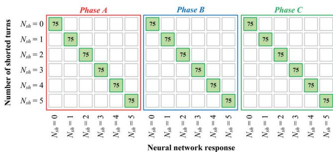
Fig. 11. Convolutional neural network response – CNN-2:  $N_{sh}$  – number of shorted turns in the individual phases; green envelope – correct neural network responses
