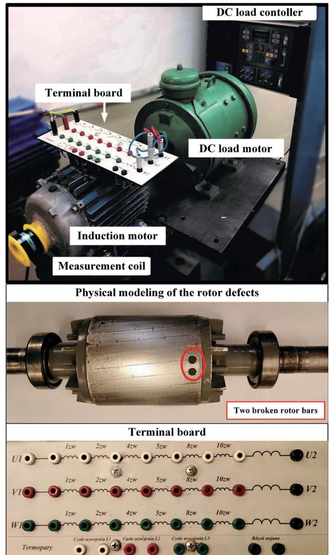
Fig. 7. Experimental set-up – real view
