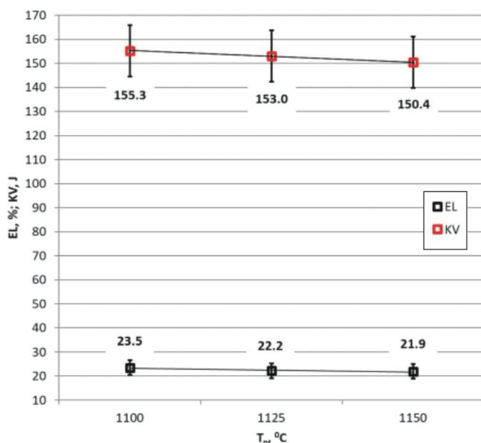
Fig. 3. Influence of hyperquenching temperature  $T_p$  on average elongation EL and impact energy KV of duplex cast steel GX2CrNiMoCuN 25-6-3-3 grade
