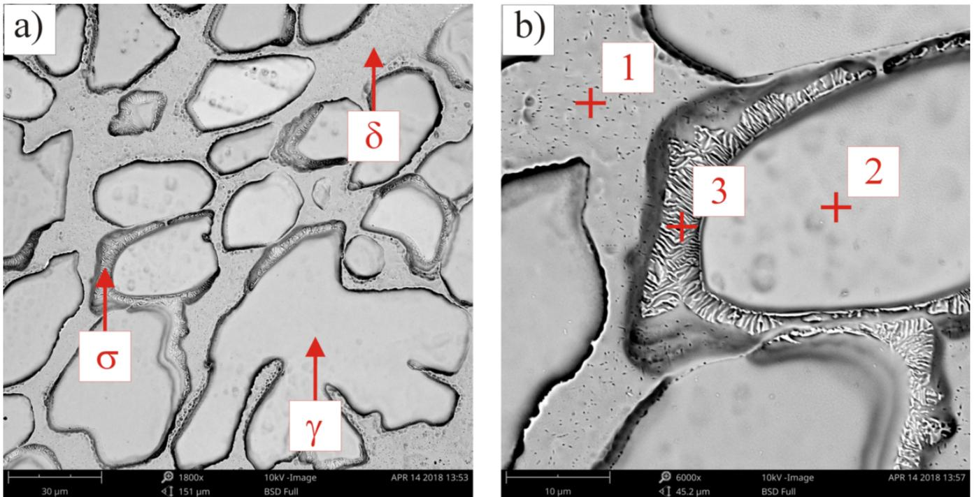
Fig. 4. Example microstructures of duplex cast steel GX2CrNiMoCu25-6-3-3 grade (melt no. 1) in as-cast state –  $\delta$  ferrite,  $\gamma$  austenite and intermetallic  $\sigma$  phase: a) SEM, mag. 800 $\times$ , b) SEM, mag. 6000 $\times$ ; 1,2 and 3 points of EDS analysis
